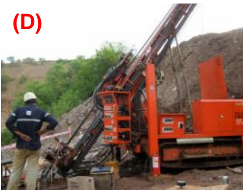
Inner tube is lowered with orientation tool & Drilling Commences
