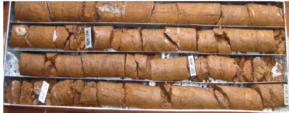
Core recovery in soft weathered formation: After
