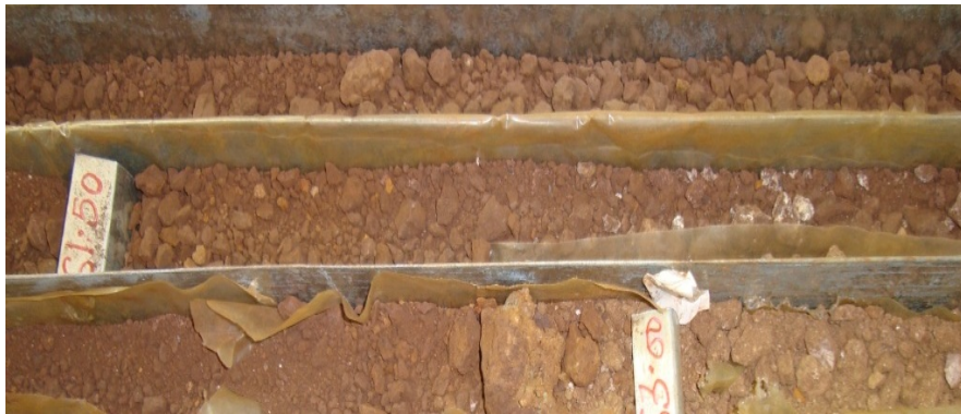
Core recovery in soft weathered formation: Before
