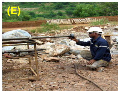
After drilling, Synchronization of the tool and Controller and Realigning
