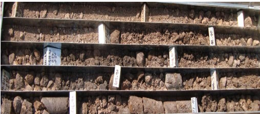
Core recovery in Friable ore: Before
